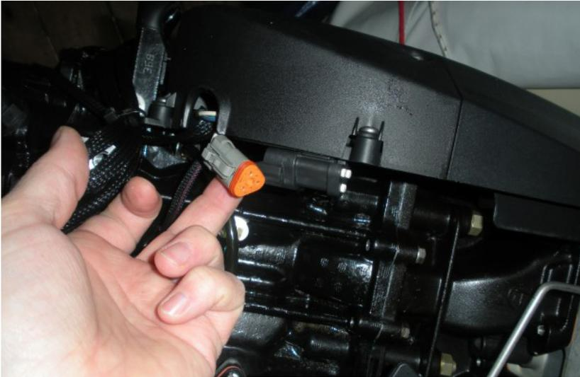
2. Remove the connector from the protective cap, and plug the Candoopro Evinrude adapter cable connector into the mating connector on the engine.
