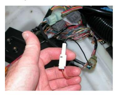
6. Insert a Kawasaki key (either FAST or SLO) into the key switch to power up the ski, ensure the emergency lanyard is attached to the stop switch, and you are now ready to start the diagnostic session.
