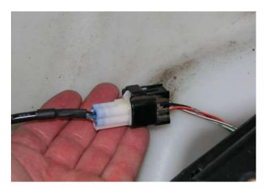
3. To keep the ECU powered up for the diagnostic session, you must attach the Immobilizer Bypass cable. The connector for the immobilizer is located behind the ECU, so you need to first remove the ECU cover panel in the front storage compartment:
