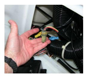
5. Disconnect this connector and connect the Late Immobilizer Bypass cable in-line:
