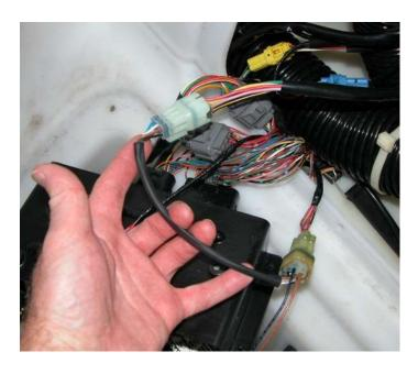
6. Once the Immobilizer Bypass cable is installed, connect the two small white one-pin connectors together on this cable:
