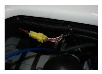
2. Remove the dust cap from the diagnostic connector, and attach the STX-1100 DI Main Diagnostic cable to the yellow diagnostic connector on the ski.
