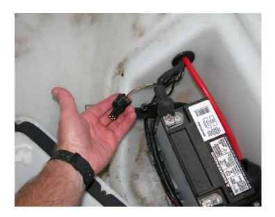
2. Remove the dust cap from the connector, and attach the Main Diagnostic cable to the diagnostic connector. NOTE: On 2007-2009 models, the Main cable connects directly to the connector on the ski. On 2010 models, you must first attach the 2010+ Adapter cable to the Main cable, then connect the 2010+ Adapter cable to the diagnostic connector on the ski.
