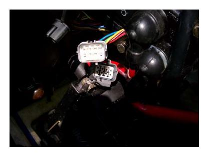
4. Disconnect the Main Relay connector and connect the Early Relay Bypass cable inline between the two halves of the Main Relay connector. Fasten the ring terminal of the Early Relay Bypass cable to the negative/ground (-) post of the battery:
