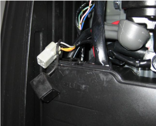
2. Remove the rubber protective cover on the connector, and plug the Candoopro Suzuki adapter cable connector into the mating connector on the engine.
