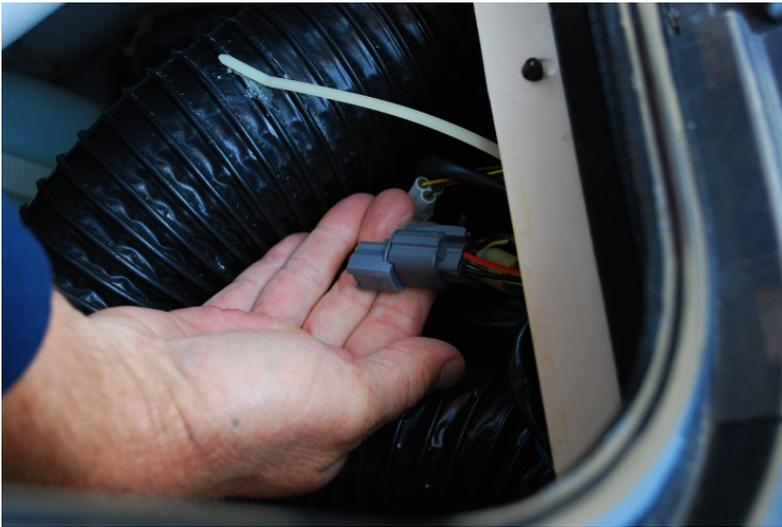
2. Disconnect this connector, and plug the Candopro Yamaha adapter cable light gray connector into the mating connector on the Waverunner harness:
