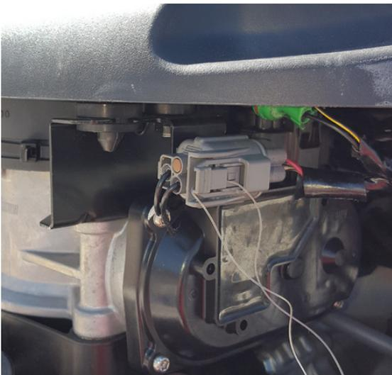
2. Disconnect this connector, and plug the Candoopro Yamaha adapter cable light gray connector into the mating connector on the Outboard harness.
